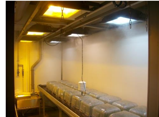
Growth chamber with 9 lamps : 6 HQI + 3 NaT, Rémi Gardet 2014
